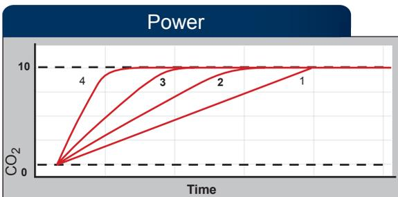
Power is a function of infusion rate of control gas. The higher the infusion rate, the faster to setpoint. Above: infusion rate #4>#3>#2>#1. Infusion rate is a function of control gas supply pressure. The higher the pressure, the higher the infusion rate. Maximum 25 PSIG provides 35 SCFH.
