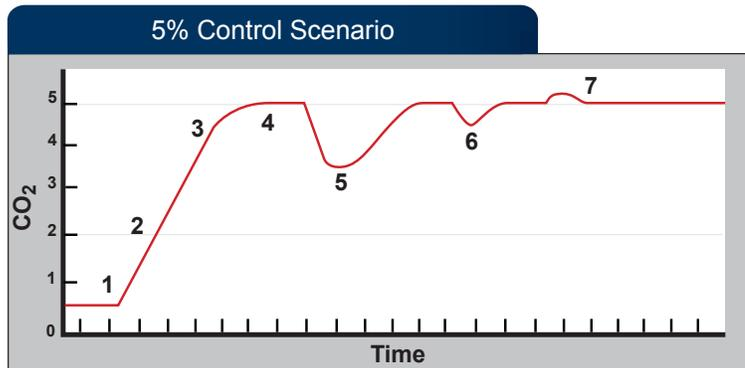
1. No control yet. Chamber CO<sub>2</sub> is ambient air CO<sub>2</sub> (0%).
