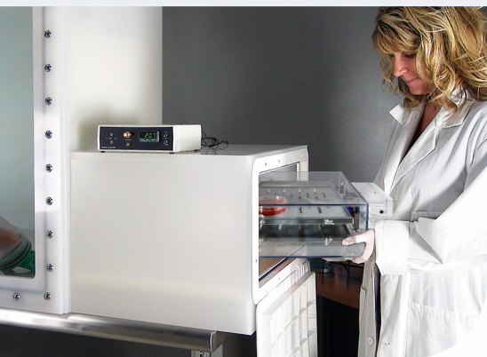
Cells are brought into the C-Shuttle via sub chamber. The buffer chamber matches the workspace environment, then cells are accessed from the interior door.
