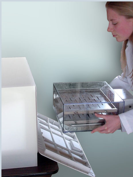
Top Left: Cultures can be handled inside the workspace at the same O_2 and/or CO_2 by simply opening the C-Chamber from inside.
