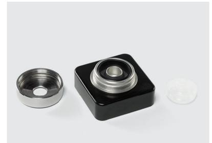
**Figure 2.** The rotor stand, molded to the shape of the rotor, supports the rotor while it is being loaded and unloaded, and immobilizes the rotor base while the rotor is being screwed on or off.
