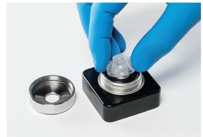
**Figure 3.** The base of the rotor is designed to completely support both chambers of the liner during centrifugation.
