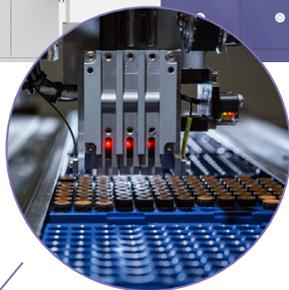
The Acoustic tube selector is tested for robustness with extensive pick and place cycles. It will pick and place three tubes at the same time for increased throughput and has been developed alongside the acoustic sample tube.
