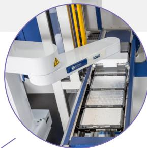
The AIM delivers samples on either an Azena High Density (HD) Tray, or more commonly on an Azena six position SBS rack tray, on its external diving board location. Any samples that can be presented onto SBS format racks (whether tubes, vials or plates) can be interchanged in this manner. This system is compatible with 96, 384, and 1536 plate formats.
