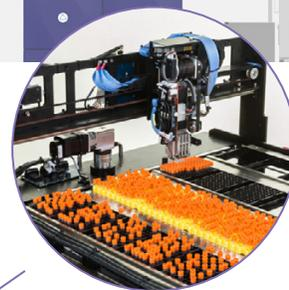
A four-lane selector allows a return order to be reformatted back into high-density storage trays and at the same time as cherry picking an order for output on the same picker. This will reduce order processing time and improve the efficiency of the store.
