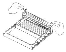
Remove the gel tray with the gel from the stand and place it into the migration tank in the correct orientation. (DNA samples will migrate from the – to + electrode.
