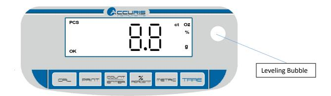
The display on the balance has a backlight, and an internal timer will turn off the backlight (power-save mode) if the balance is not used for a period of time. The default time delay for back light shut off is one minute, and this time is adjustable by following these instructions:
