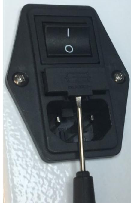
2. Replace fuses as required with 250V 10A fuses. Close fuse panel.
