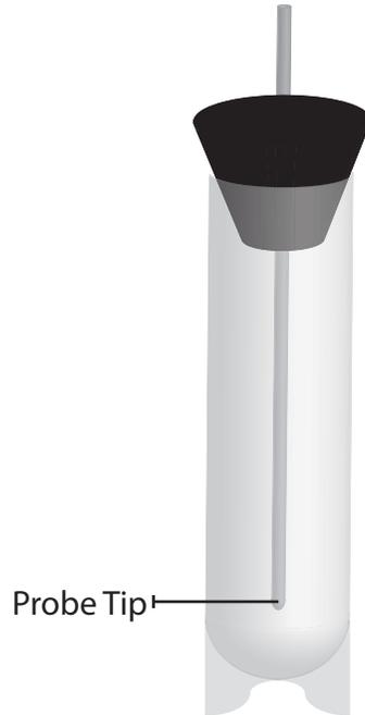
Probe tip must be equal distance from each side of the vial and from the bottom of the vial.
