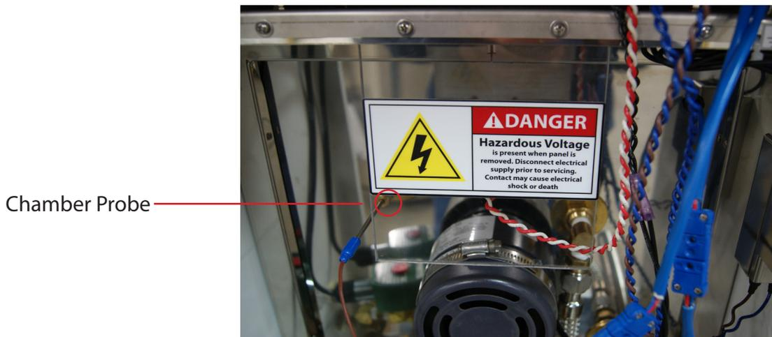
9. Locate and replace the chamber probe by tightening the brass fitting using 3/8" wrench. [F]
