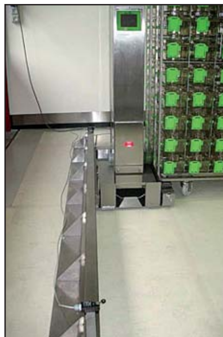
Picture 2: library runs along a rail to fix the direction of movement.
