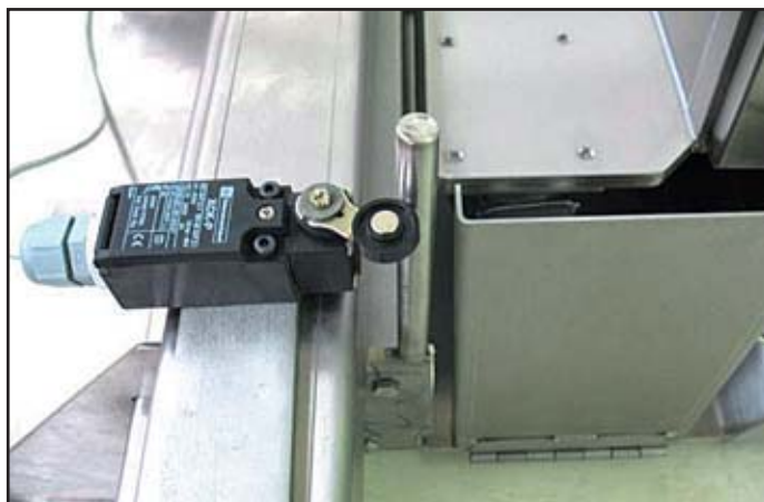
Picture 3: end run interrupter to invert direction and count cycles.
