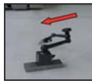
Picture 5: analogical comparator used to measure deformations in the vinyl floor due to platform movements. The red arrow shows an imprint left by the castors.
