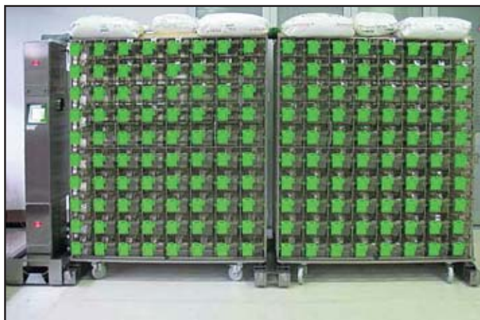
Picture 1: library configuration used in the test. It is composed of 2x2GM160 racks, an Air Handling Unit, the lifting platform and a load to simulate animals, bedding, food and water. The system moves along a vinyl floor.
